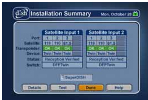
Figure 9. DISH Pro Plus Installation Summary
