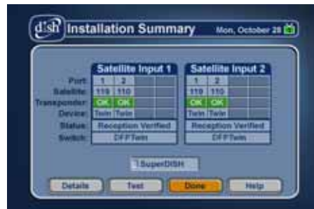
Figure 7. DISH Pro Plus Installation Summary
