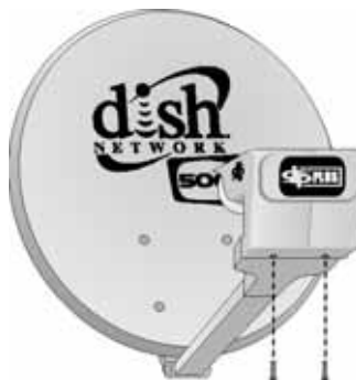
Figure 2. Connecting DISH Pro Plus Twin to DISH 500 Y-Bracket and Cabling
